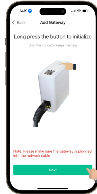
05. Press and hold the initialization key to enter initialization status, the indicator light will flash, then click Next.
